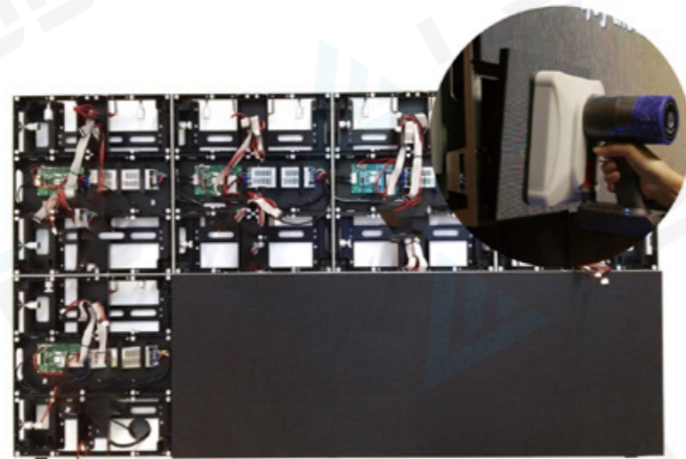
Step 4: Connect the power cable and data cable on modules first, then use vacuum tool to put the modules on cabinet. In this process, can adjust the screen flatness.
